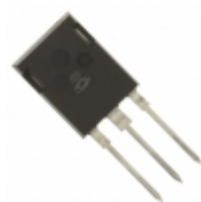
APT56F60B2 Microsemi Corporation MOSFET N-CH 600V 60A TO-247
