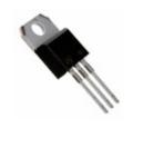
**BUL49D** STMicroelectronics TRANS NPN 450V 5A TO-220
