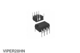
STMicroelectronics IC OFFLINE CONV PWM OVP 8DIP
