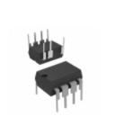
VIPER27HN STMicroelectronics IC OFFLINE CONV PWM OVP 7DIP
