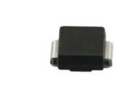
SM6T82CAY STMicroelectronics TVS DIODE 70VWM 146VC SMB
