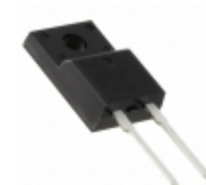
DPG15I400PM IXYS DIODE GEN PURP 400V 15A TO220FP
