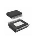
L9960T STMicroelectronics IC HALF-BRIDGE DRVR SPI PWRSSO36
