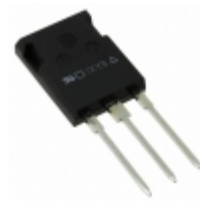
DSEP75-06AR IXYS DIODE GEN 600V 75A ISOPLUS247
