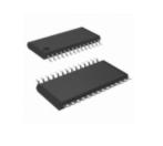
IDT5V2528APGGI8 IDT (Integrated Device Technology) IC CLK DVR ZD BUFFER PLL 28TSSOP
