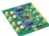
AD8335-EVALZ ADI (Analog Devices, Inc.) BOARD EVALUATION FOR AD8335
