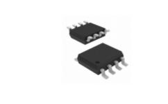
AOZ1014AI Alpha and Omega Semiconductor, Inc. IC REG BUCK ADJ 5A 8SOIC
