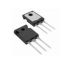
**STGWA15S120DF3** STMicroelectronics IGBT 1200V 15A TO247-3L
