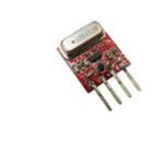
**QAM-TX2-433 RF Solutions** MODULE AM TRANSMITTER
