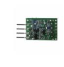
**QAM-TX1-433** RF Solutions TRANSMITTER MOD AM 433MHZ
