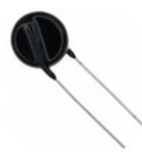
ERZ-V20D431 Panasonic Electronic Components VARISTOR 430V 10KA DISC 20MM
