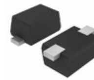
EDZTE616.2B Rohm Semiconductor DIODE ZENER 6.2V 150MW EMD2
