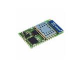
SPWF04SC STMicroelectronics WIFI MODULE WITH U.FL. CONNECTOR
