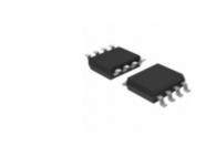
**ALD910016SAL** Advanced Linear Devices Inc. MOSFET DUAL SAB 10.6V EE 8SOIC
