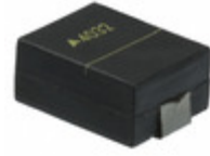
CU4032K175G2 EPCOS (TDK) VARISTOR 270V 1.2KA 4032
