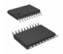
CY2CP1504ZXC Cypress Semiconductor Corp IC CLK BUFFER 2:4 250MHZ 20TSSOP
