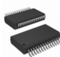
PIC16C72T-04E/SS Micrel / Microchip Technology IC MCU 8BIT 3.5KB OTP 28SSOP
