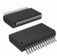
PIC18LF24J50-I/SS Micrel / Microchip Technology IC MCU 8BIT 16KB FLASH 28SSOP
