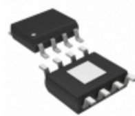
SPA-2118Z RFMD IC AMP HBT GAAS 850MHZ 8-SOIC
