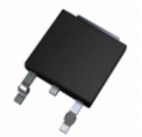
IXTY02N120P IXYS MOSFET N-CH 1200V 0.2A DPAK
