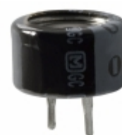
EEC-F5R5H104 Panasonic Electronic Components CAP 100MF -20% +80% 5.5V T/H
