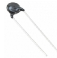
ERZ-E07A471 Panasonic Electronic Components VARISTOR 470V 2.5KA DISC 9MM
