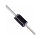
1N5404G-T Diodes Incorporated DIODE GEN PURP 400V 3A DO201AD
