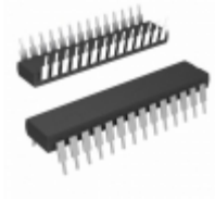
PIC16C72-04E/SP Micrel / Microchip Technology IC MCU 8BIT 3.5KB OTP 28SDIP
