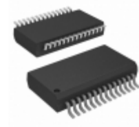
PIC16C72AT-20I/SS Micrel / Microchip Technology IC MCU 8BIT 3.5KB OTP 28SSOP
