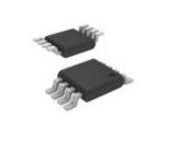
PI90LV017AUEX Diodes Incorporated IC LVDS DIFF LINE DVR 3V 8-**MSOP**
