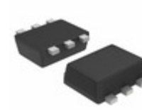
EMZ1DXV6T1 ON Semiconductor TRANS NPN/PNP 60V 0.1A SOT563
