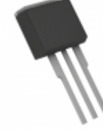
IRF3704LPBF International Rectifier (Infineon Technologies) MOSFET N-CH 20V 77A TO-262
