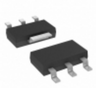
NCV1117ST33T3 AMI Semiconductor / ON Semiconductor IC REG LDO 3.3V 1A SOT223
