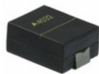
CU4032K11G2 EPCOS (TDK) VARISTOR 18V 250A 4032
