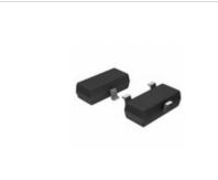
**STM1817TWX7F** STMicroelectronics IC RESET CIRCUIT 3.06V PP SOT-23
