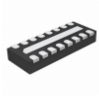
PEMI8QFN/HG,132 NXP Semiconductors / Freescale FILTER RC(PI) 45 OHM/11PF SMD
