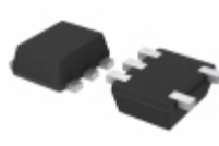
BU4828FVE-TR LAPIS Semiconductor IC VOLT DETECTOR STD 5-VSOF
