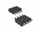
**M24SR64-YMN8T/2** STMicroelectronics IC NFC/RFID TAG 64KB EEPROM 8SOI
