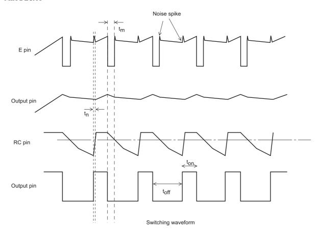
ton: Output ON time toff: Output OFF time
