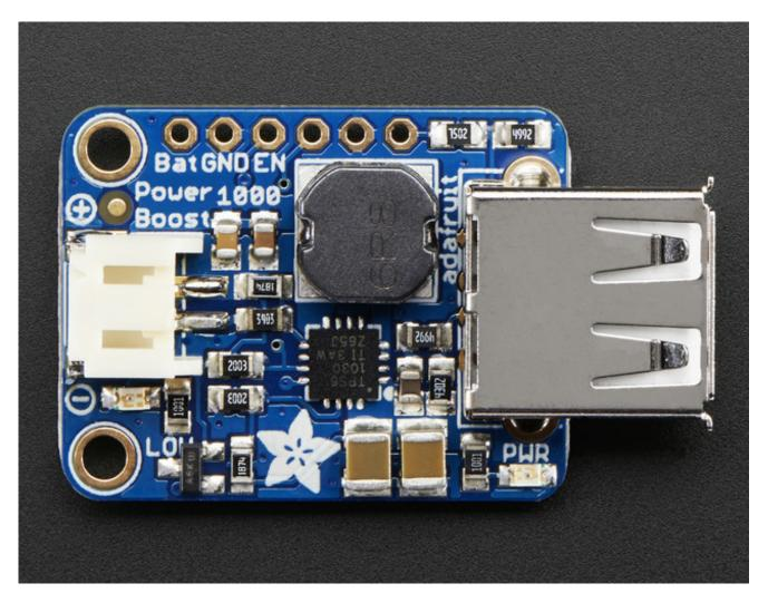
The PowerBoost 1000 has at the heart a TPS61030 boost converter from II (http://adafru.it/dLY). This boost converter chip has some really nice extras such as low battery detection, 4A internal switch, synchronous conversion, excellent efficiency, and 700KHz high-frequency operation. Check out these specs!
