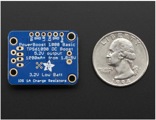
Great for powering your robot, Arduino project, single-board-computer such as Raspberry Pi or BeagleBone! Each order comes with one fully assembled and tested PCB, a loose 2-PH JST jack, a 2-pin Terminal block and a loose USB A jack.
