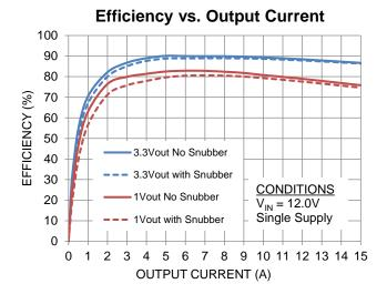
Figure 11: Efficiency with/without Snubber
