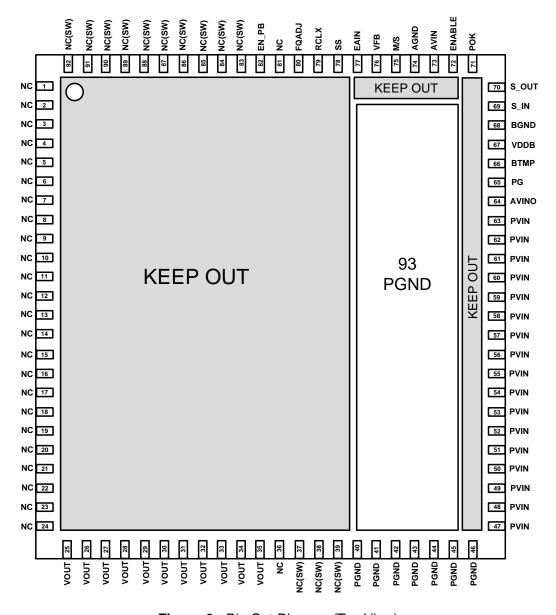
Figure 3: Pin Out Diagram (Top View)
