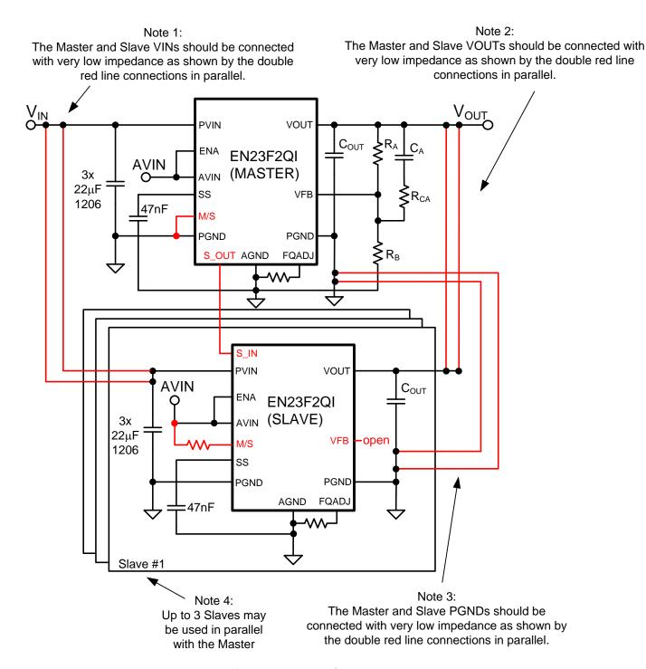
Figure 9. Parallel Operation Illustration
