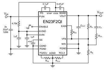
Figure 5: Single Input Supply Schematic
