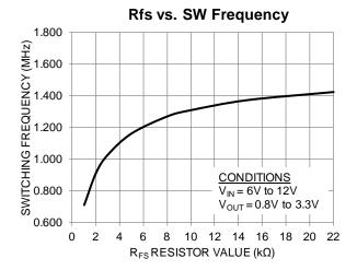
**Figure 7**. R<sub>FS</sub> versus Switching Frequency
