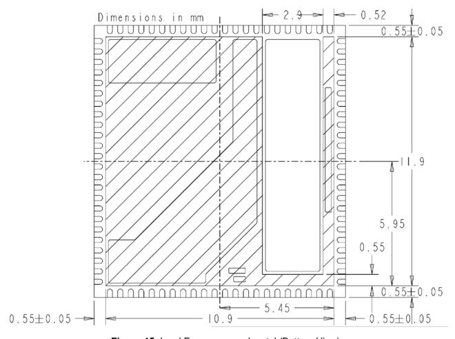
Figure 15: Lead-Frame exposed metal (Bottom View)
