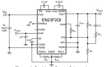
Figure 6: Dual Input Supply Schematic
