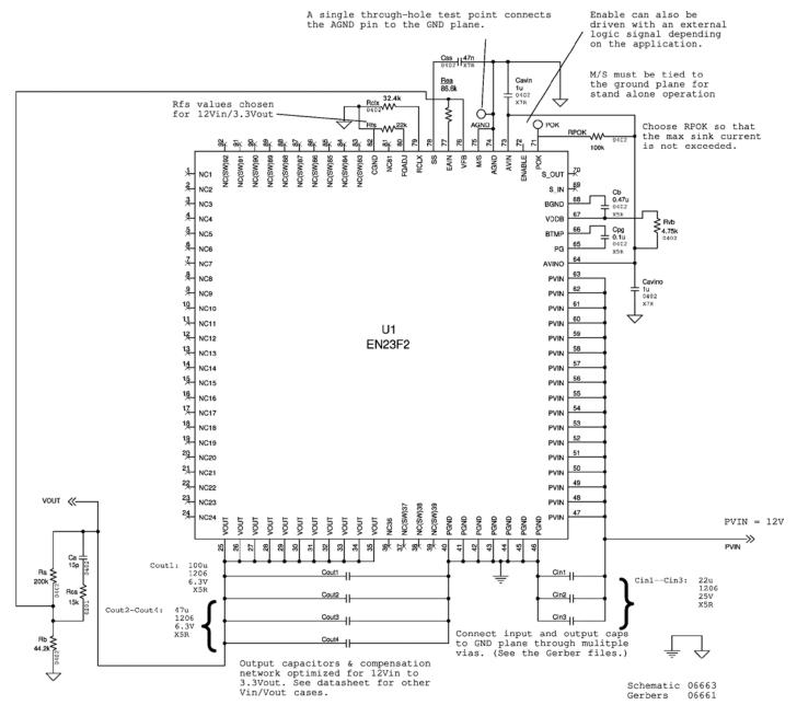
Figure 13: Engineering Schematic
