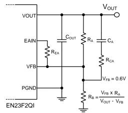
**Figure 10:** V<sub>OUT</sub> Resistor Divider & Compensation Components. See Table 4 for details.
