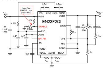
Figure X. Pre-Bias Application Circuit
