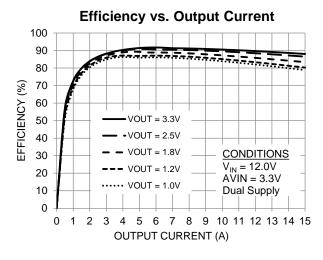
Figure 12: Efficiency vs. Output Current For  $V_{IN} = 12V$ ,  $V_{OLIT} = 1.2V$  at 15A,  $\eta \approx 80\%$
