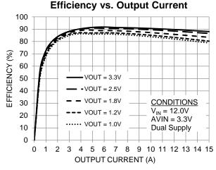
**Figure 2.** Highest Efficiency in Smallest Solution Size
