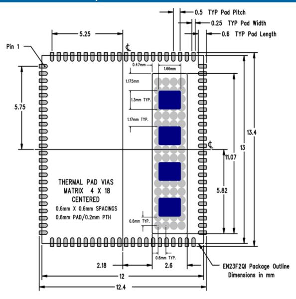
Figure 16: EN23F2QI PCB Footprint (Top View)
