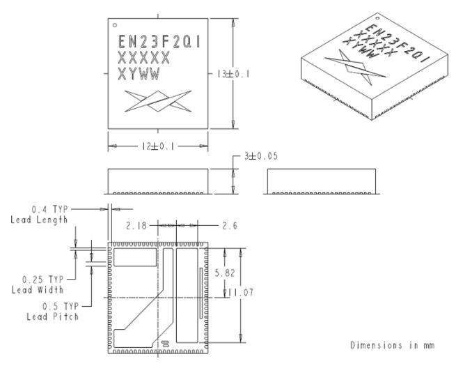
Figure 17: EN23F2QI Package Dimensions (Bottom View)
