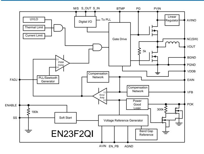
Figure 4: Functional Block Diagram
