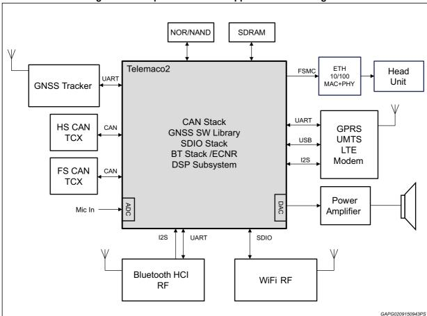
Figure 1. Example of telematics application block diagram
