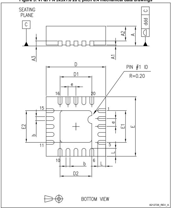
Figure 5. VFQFPN 3x3x1.0 20 L pitch 0.4 mechanical data drawings
