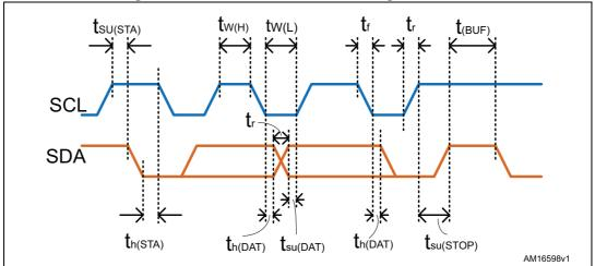
Figure 3. SMBus communication timing waveforms
