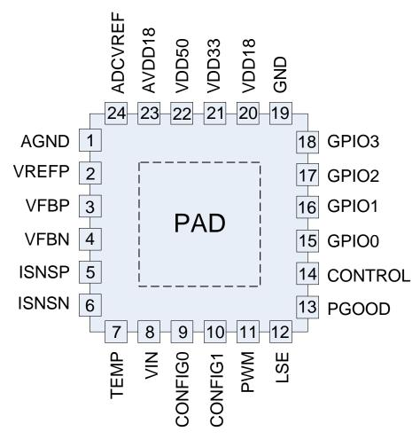
Figure 2: Pin Out Diagram (Top View)
