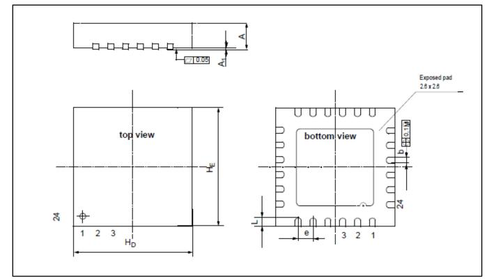
Figure 7: 24-pin QFN Package Drawing
