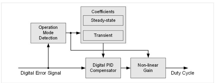
Figure 4: Simplified Block Diagram for the Digital Compensation
