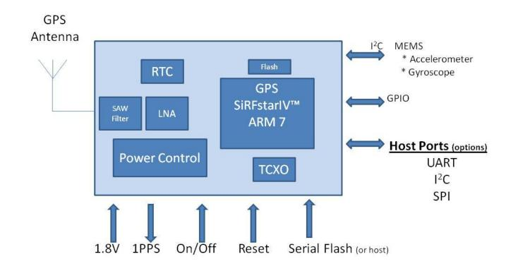
Figure 1 Inventek's ISM420R1-CX General Block Diagram
