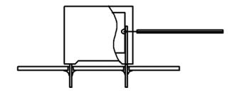
Temperature monitored inside the capacitor.
