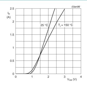
$T_j$  = 25 °C and 150 °C;  $V_{DS} > I_D \times R_{DSon}$
