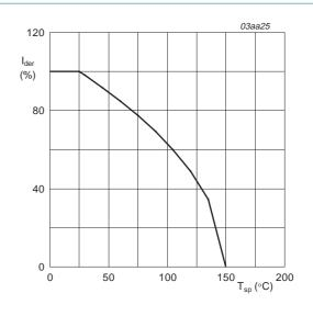
$$I_{der} = \frac{I_D}{I_{D(25^{\circ}C)}} \times 100 \%$$
