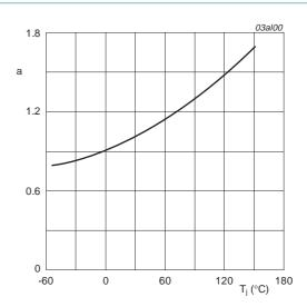
$$a = \frac{R_{DSon}}{R_{DSon(25^{\circ}C)}}$$
