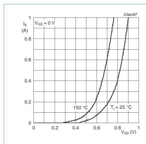
$T_j$  = 25 °C and 150 °C;  $V_{GS}$  = 0 V
