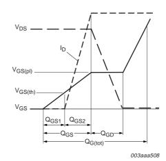
Fig 12. Gate charge waveform definitions
