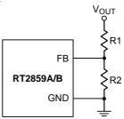
Figure 4. Output Voltage Setting
