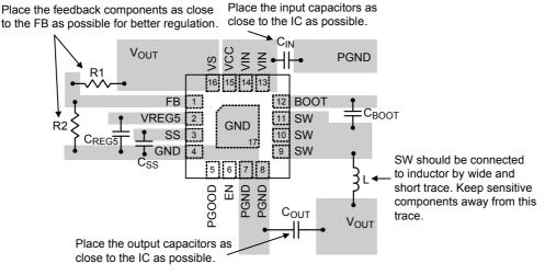
Figure 2. PCB Layout Guide
