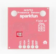
Addresses 0 and 1 can be used to change the I<sup>2</sup>C address of the board in case you have multiple devices using the same address. The below table shows the addresses that correspond to the different combinations of opened and closed jumpers.
